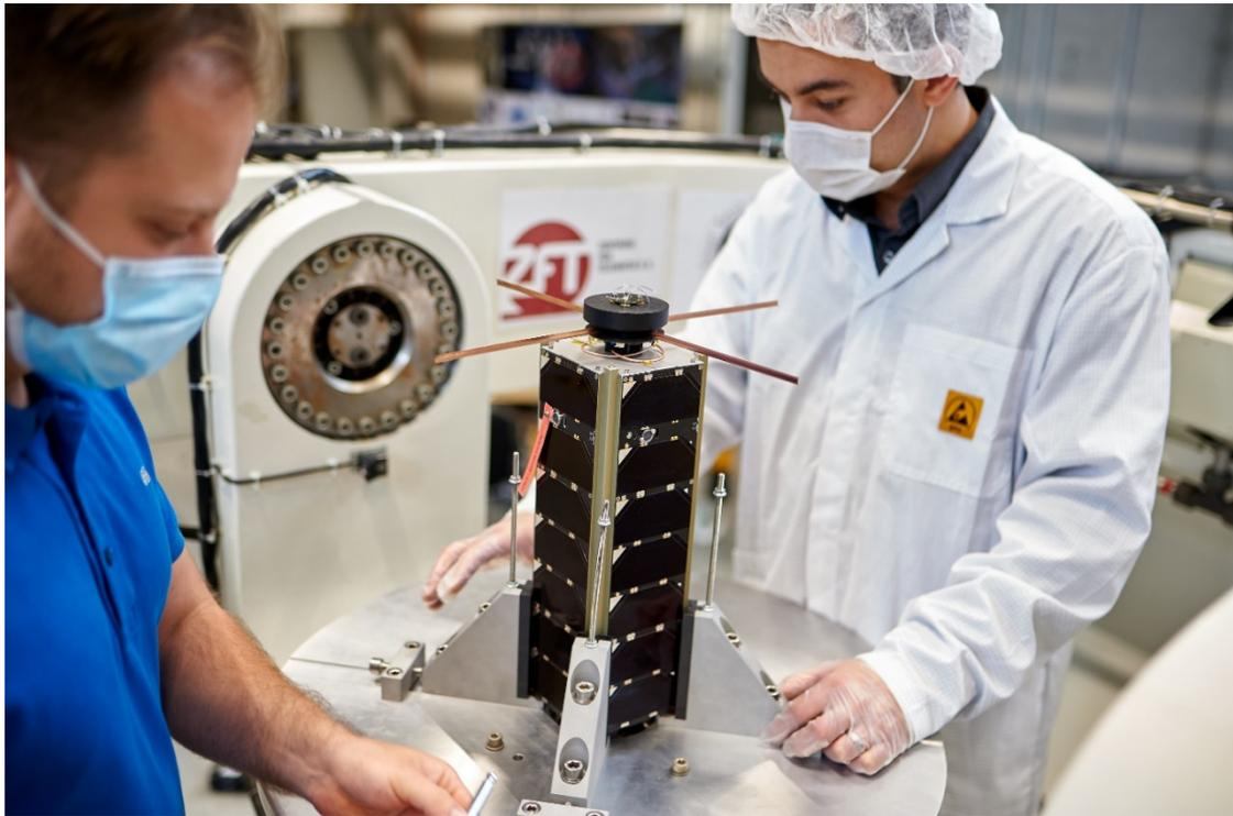
Preparation of a NetSat satellite for testing on an extremely dynamic turntable
