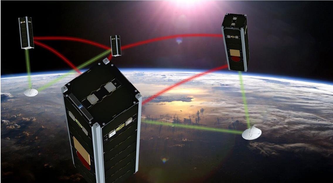
NetSat: 4 nano-satellites with dimensions 10 cm x 10 cm x 30 cm for formation flight in an orbit at 600 km altitude (source: ZfT).
