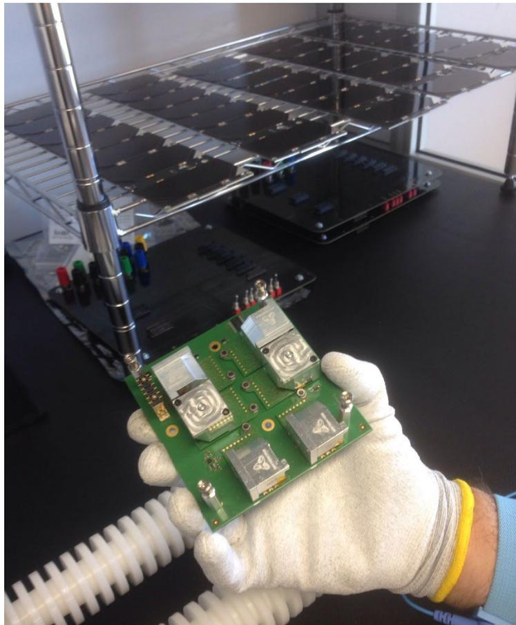
The attitude control system, composed of 6 miniature reaction wheels, guaranteeing by redundant components extreme robustness as well as precision pointing of the satellite. In the background the sidepanels equipped with are stored (source: ZFT).
